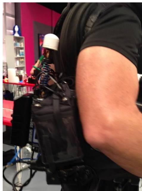
5.8 GHz 3 dBi Gain Omni-directional Antenna directly against the back of the Cinematographer
