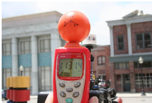
Field intensity measurement of COFDM Camera Back Wireless Video Transmitter at Golden Oak Ranch.
